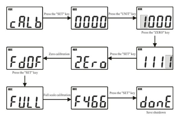
7.10 Restore factory settings: This setting is convenient for users to set up confusion, and can restore the factory settings with one key. Enter the system menu, select this setting and press the "SET" key to restore the factory settings, the instrument automatically shuts down. If you continue to use the instrument and press the power button, the instrument has been restored to the factory default settings.
