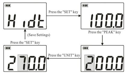
7.2 Measured value lower limit: Set the measured value lower limit. The lower limit value is 0 by default. If the measured value is lower than the lower limit, it is out of range. The screen displays "MIN" and the buzzer sounds long. The user can freely set the lower limit value, select this menu to set the value, the operation steps are the same as the upper limit value.
