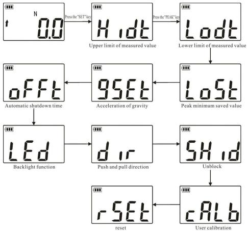
7.1 Upper limit of measured value: Set the upper limit of the measured value. The upper limit is the full range by default. The measured value is higher than the upper limit and is out of range. The screen displays "MAX" and the buzzer alarm sounds for a long time. As shown below:
